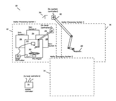
(57) Abstract: The invention provides, in some aspects, a wafer alignment system comprising an image acquisition device, an illumination source, a rotatable wafer platform, and an image processor that includes functionality for mapping coordinates in an image of an article (such as a wafer) on the platform to a "world" frame of reference at each of a plurality of angles of rotation of the platform.
