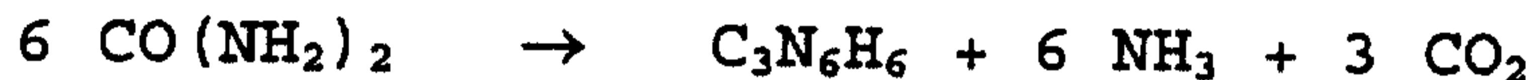
The preparation can be carried out at a high 10 pressure, preferably between 7 and 25 MPa, without the presence of a catalyst. The temperature of the reaction varies between 325 and 450°C and is preferably between 370 and 440°C. The NH<sub>3</sub> and CO<sub>2</sub> byproducts are usually returned to an adjoining urea plant.
