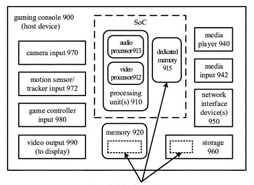
software 930 implementing one or more innovations for virtualizing audio decoding hardware of a guest device by a host device
