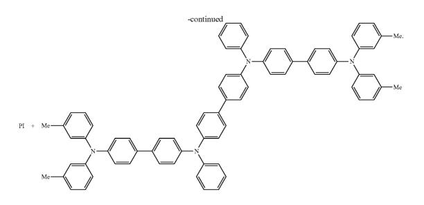
**[0044]** According to another embodiment the resistively switching material is an endcapped polyfluorene of the following formula without being restricted thereto:
