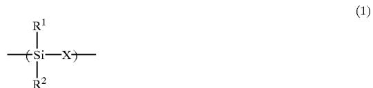
[0013] wherein  $\text{R}^1$  and  $\text{R}^2$  each represent an optionally substituted alkyl, alkoxy, aryl or aryloxy group; and  $\text{X}$  represents an oxygen atom, a nitrogen atom, an alkylene group, a phenylene group, a silicon atom, a metal atom or an atomic group in combination thereof.
