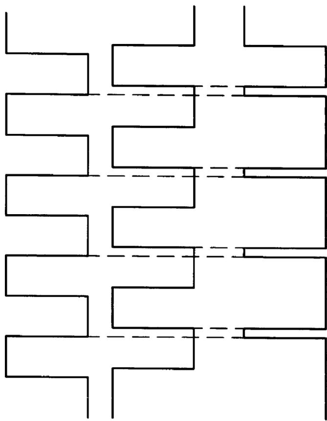
OUTPUT SIGNAL OF RING OSCILLATOR
