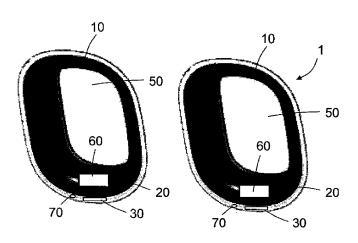
(57) Abstract: The present invention provides a window module for an aircraft or spacecraft, comprising a window frame (10) which comprises, at least in portions, a current-generating element (20) for generating an electric current.
