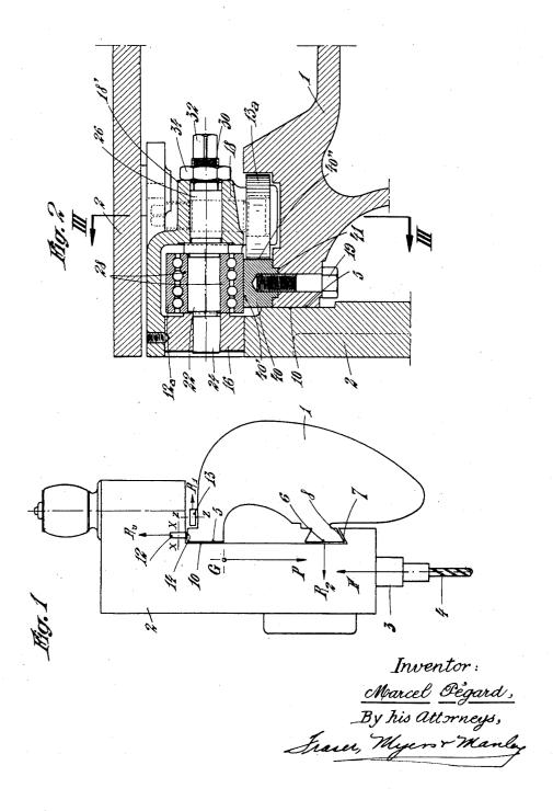
CARRIAGE CONTROL MEANS OF MACHINE-TOOLS
