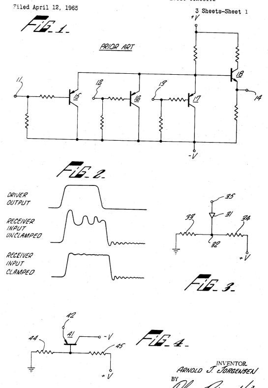
INTEGRATED ANTI-RINGING CLAMPED LOGIC CIRCUITS
