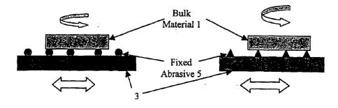
(57) **Abstract:** A plurality of nanoparticles are provided. The nanoparticles may have a metal oxide or a semiconductor oxide surface region and a metal or semiconductor core region and/or the nanoparticles may be uniformly doped. The nanoparticles are formed by grinding a bulk material to a powder and then etching the powder in a solution to a desired nanoparticle size.
