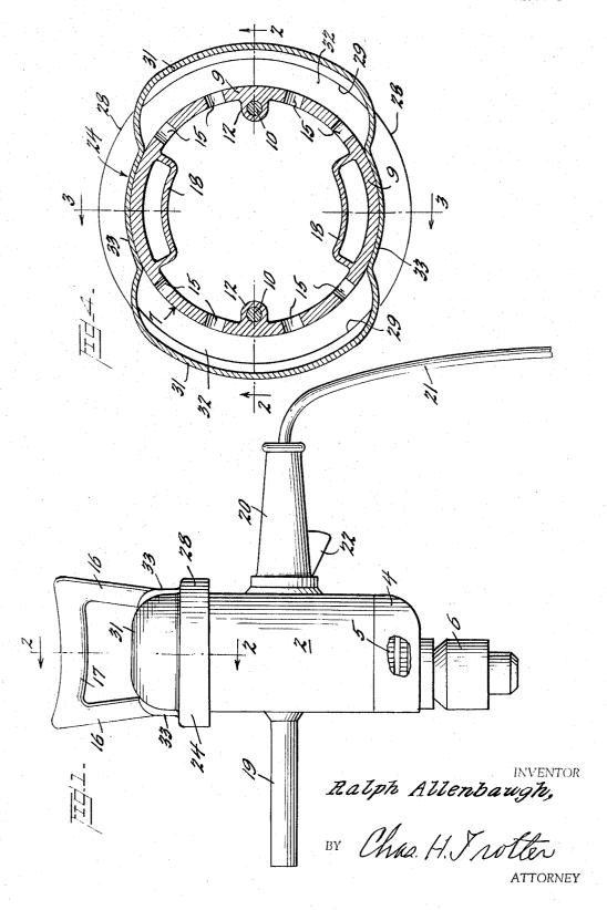
PORTABLE ELECTRIC HAND TOOL WITH A MOISTURE REPELLANT COVER
