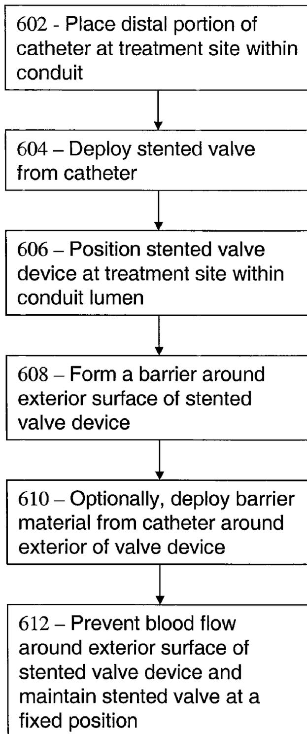
**CATHETER DELIVERED VALVE HAVING A
