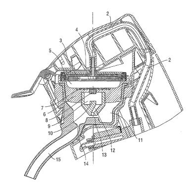
(57) Abstract: A beverage making device comprising a frothing member (9) for producing froth in the beverage, which device comprises a settling chamber (11) for settling the frothed beverage coming from the frothing member (9). The coarse foam is separated from the fine foam thereby. The outlet (14) for the settled beverage is at the lower side of the settling chamber (11).
