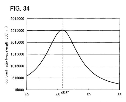
angle of absorption axis of polarizer on viewing side (deg.)
