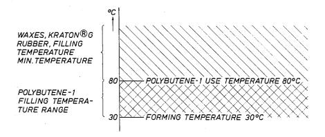
FIG.1 TEMPERATURE FILLING RANGES AND USE TEMPERATURES FOR POLYBUTENE-1, WAXES, KRATON®G RUBBER, etc
