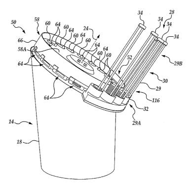
(57) Abstract: A device (Fig. 2) for sorting discs ejects the disks from the receptacle by means of a rotating wheel with numerous wells (62) into collecting devices (34).
