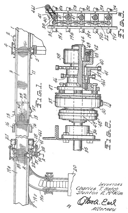
C. T. HATCH ET AL CONVEYOR SYSTEM FOR ADVANCING AND DIVIDING A SERIES OF ARTICLES 2,724,486
