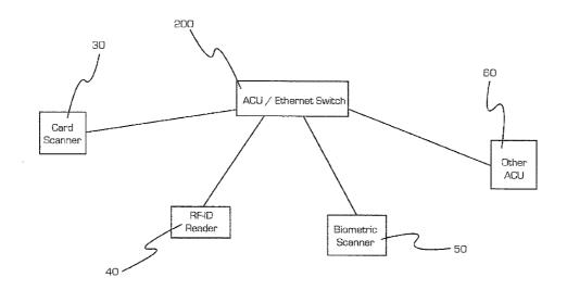
Other ACU 20 Biometric Scanner Primary Access Control Unit (P-ACU) PRIOR ART **Éthernet Routing Unit** FIG. 1 Reader RF-ID 2 30 Scanner Card
