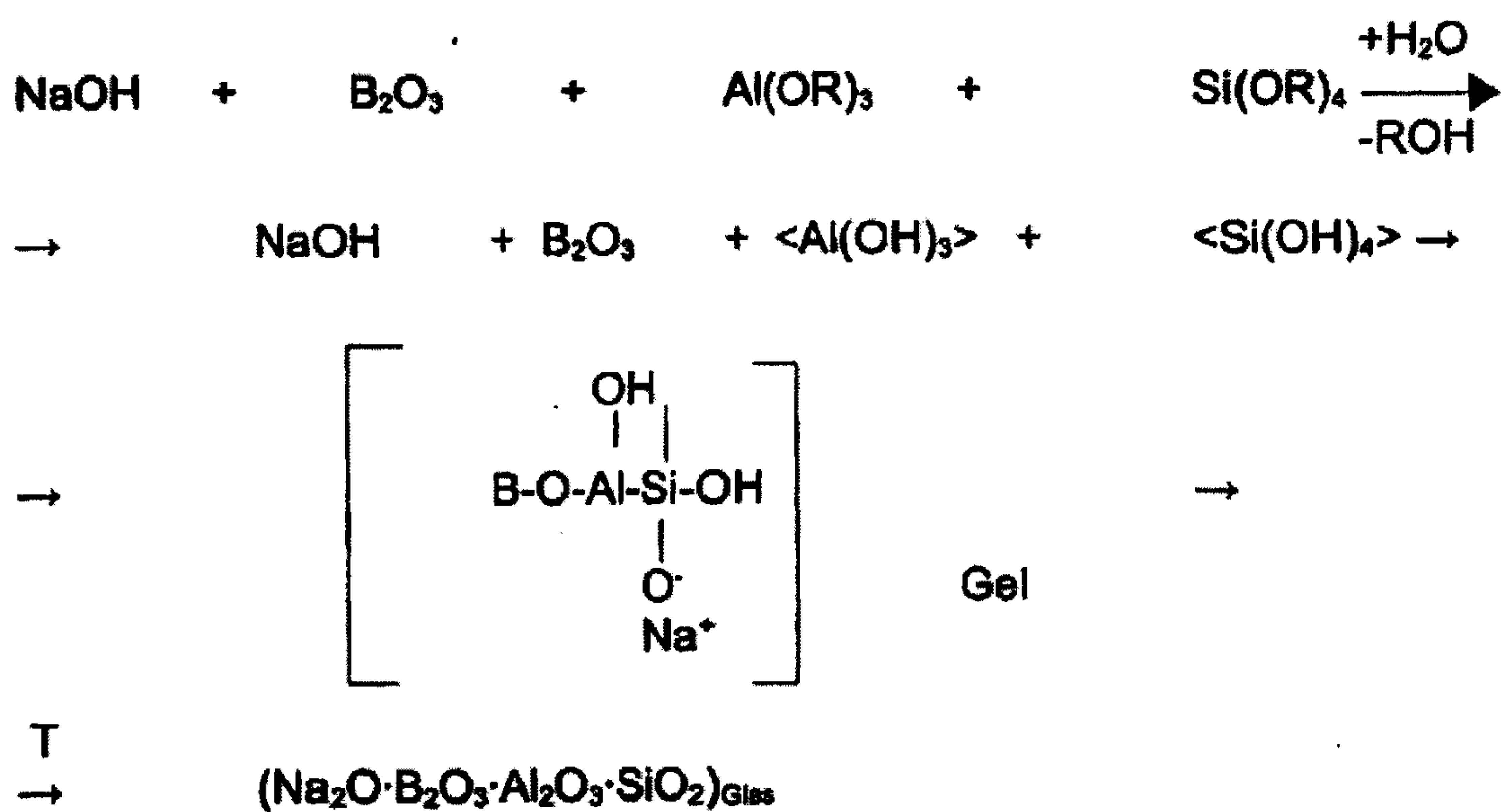
Water is added to begin the hydrolysis process of the starting components. The reaction proceeds relatively quickly because the alkali ions have a catalytic effect on the speed of hydrolysis of the silicic acid ester. Once the gel is formed it can be dried and 15 densified by means of a thermal process to form glass.
