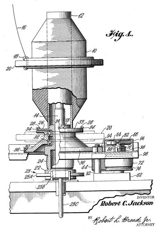
SPINNING AND TWISTING APPARATUS
