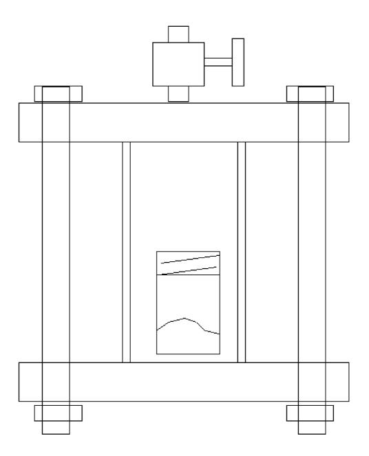
The pressure in the vessel is then released, quickly producing a foamed polymer. The blowing agent plasticizes the polymer as it dissolves into it. The resulting density of the two foams thus produced using this method is determined and found to be acceptable.
