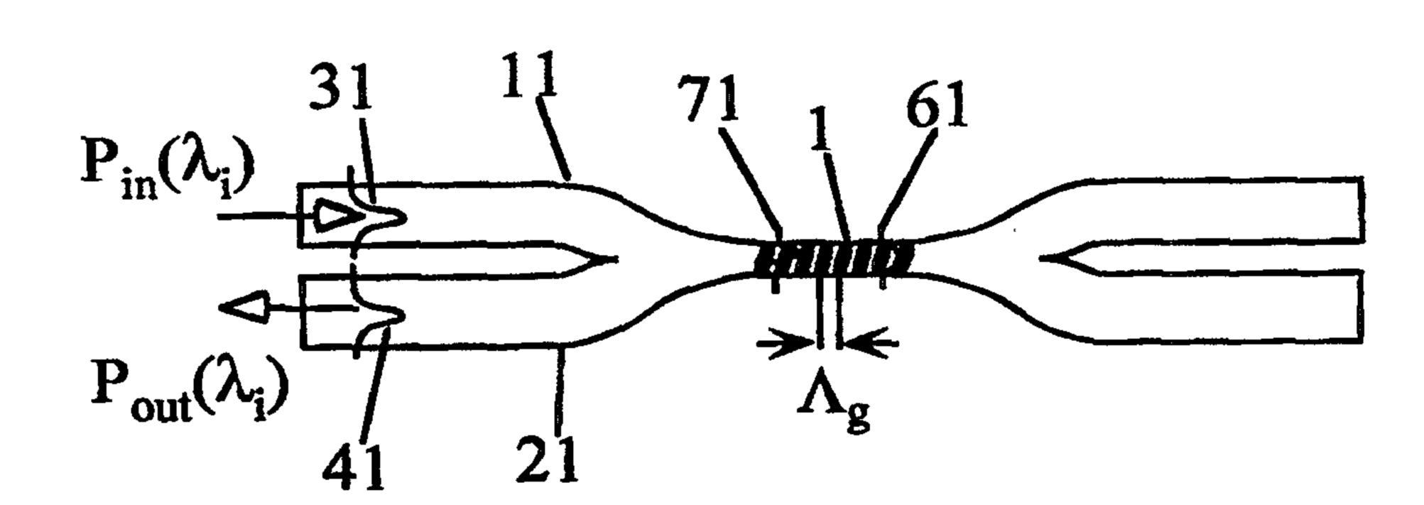
routers (5), and sources to be fabricated. The grating assisted mode coupler (23) can be wavelength tuned by modifying the optical properties of the coupler interaction region. A programmable, wavelength selective router (5) composed of multiple grating assisted mode couplers is also disclosed.
