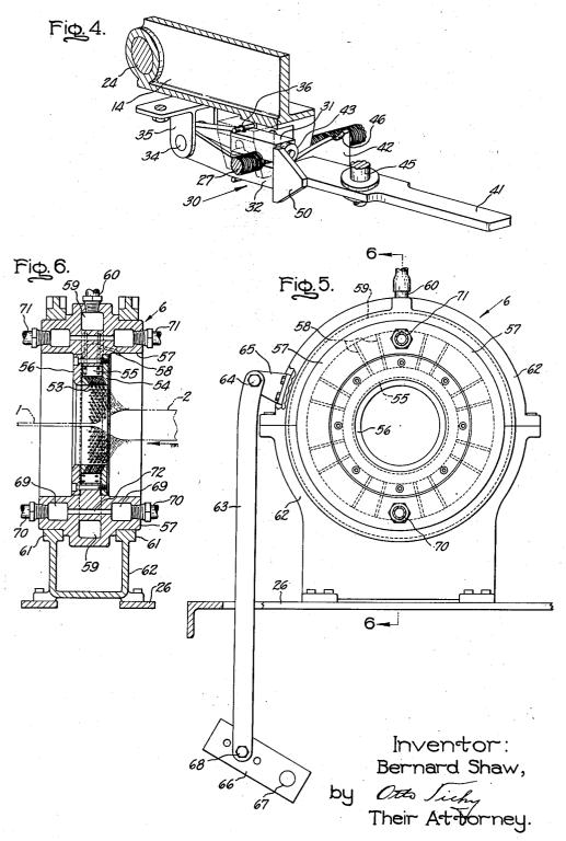
APPARATUS FOR DRAWING VITREOUS TUBES AND RODS
