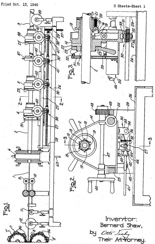
APPARATUS FOR DRAWING VITREOUS TUBES AND RODS
