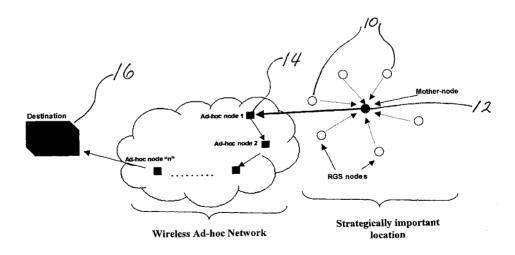
(57) Abstract: Ultra wideband radar motion sensors strategically placed in an area of interest communicate with a wireless ad hoc network to provide remote area surveillance. Swept range impulse radar and a heart and respiration monitor combined with the motion sensor further improves discrimination.
