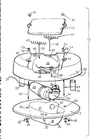
(57) Abstract: A floating pond skimmer is connected to remote filter. The skimmer includes a vortex (38), an on-board pump (32) with a grinding impeller, an adjustable ballast (52, 54) and an anchor.
