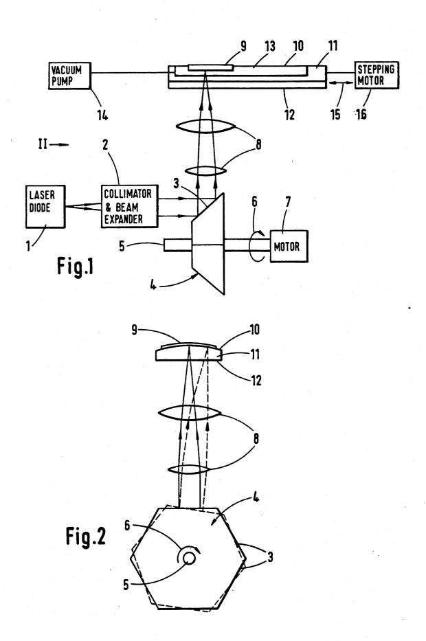
Although the polygon mirror may have any suitable plurality of facets for redirecting the radiant energy, in the preferred embodiment the mirror is hexagonal.
