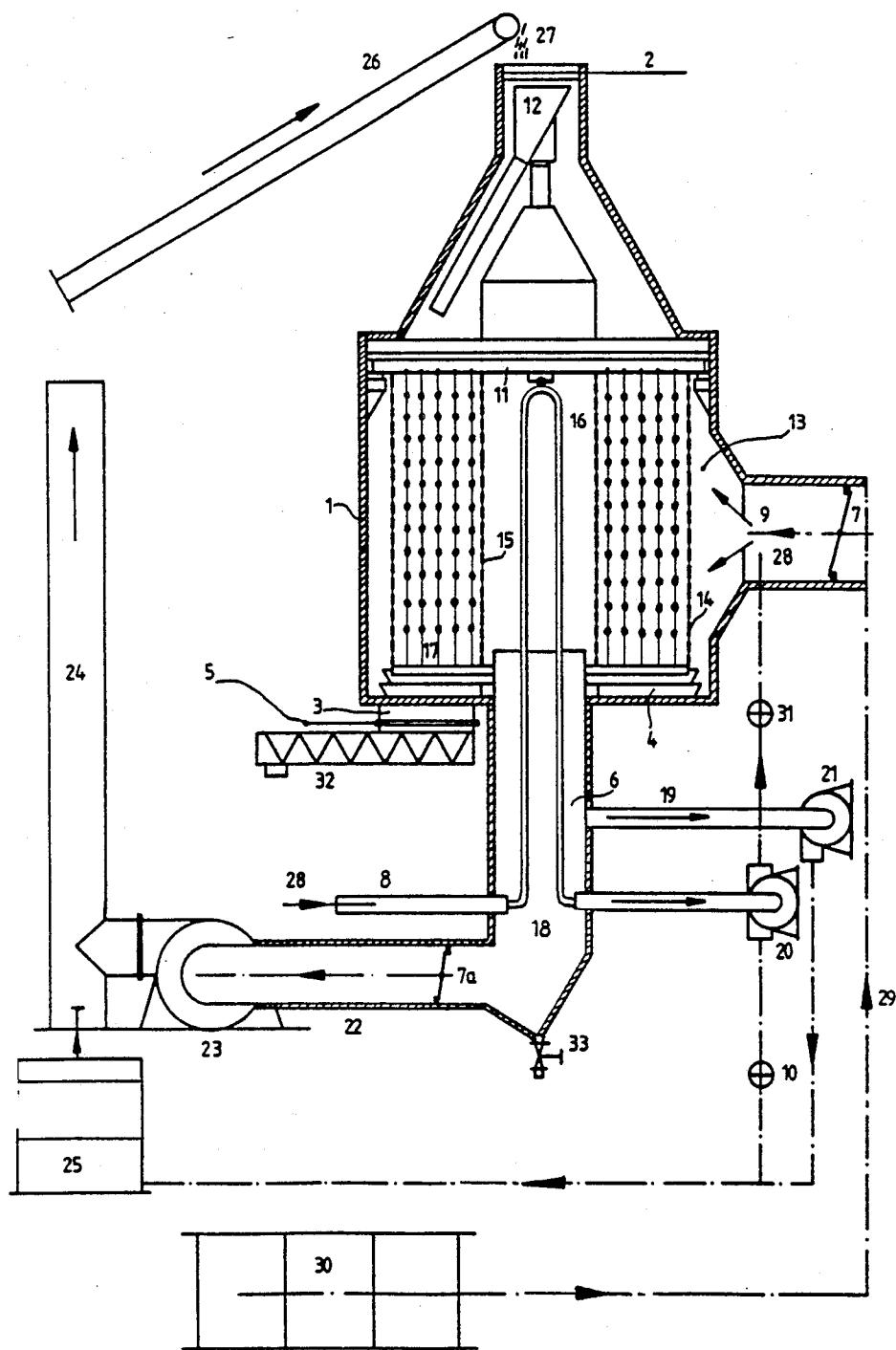
**PROCESS AND APPARATUS FOR DRYING AND CONDITIONING CHICKEN MANURE OR SIMILAR PASTY SUBSTANCES**
