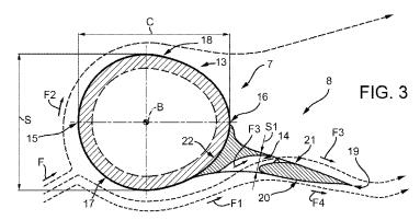
(57) Abstract: An aerodynamic appendix (8) for a wind turbine blade (7) is designed to fit to the inner portion (12) and intermediate portion (13) of the wind turbine blade (7), and has a trailing edge (19), a pressure side (20), a suction side (21), and at least one duct (14) connecting the pressure side (20) fluidically to the suction side (21).
