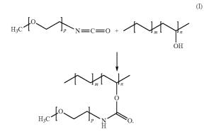
**[0023]** The conditions under which reaction scheme (I) is conducted can be determined by one having ordinary skill in the art. As a result, EVAL is firmly bonded to the biologically compatible PEG-ISO to form the urethane product of reaction scheme (I). Thus, EVAL, modified by PEG-ISO, can have an enhanced long-term biocompatibility.
