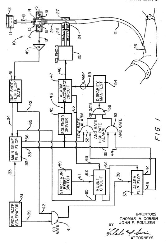
APPARATUS FOR MONITORING THE DISPENSING OF LIQUID
