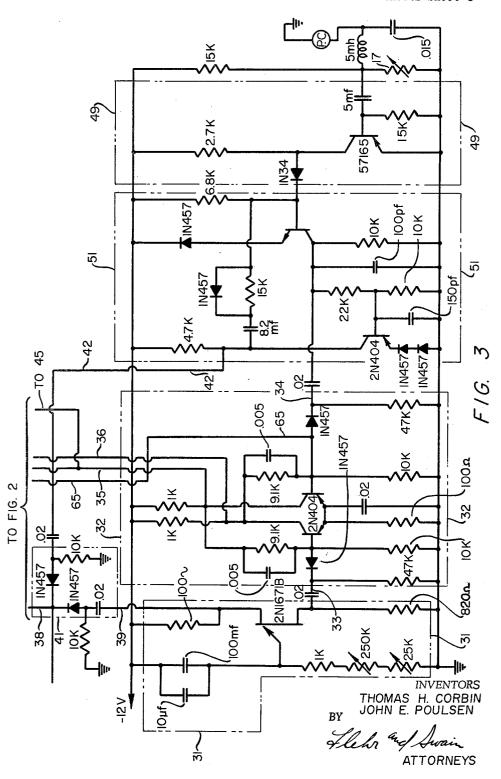
3,197,068 APPARATUS FOR MONITORING THE DISPENSING OF LIQUID
