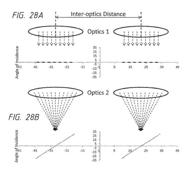
Max/Min Combined Angles of Incidence for Optics 1 and 2
