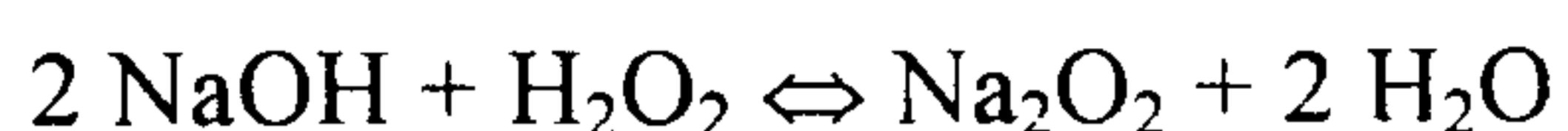
This mixture containing the sodium peroxide was then placed within a glass dropping funnel which was securely clamped above the 15 liter stainless steel beaker containing the ethyl chloroformate. The temperature within the steel beaker was 0°C. The homogenizer was running throughout the synthesis reaction to form the peroxydicarbonate.
