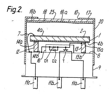
INFRARED RADIATION DETECTOR WITH INTEGRAL FRESNEL LENS WINDOW
