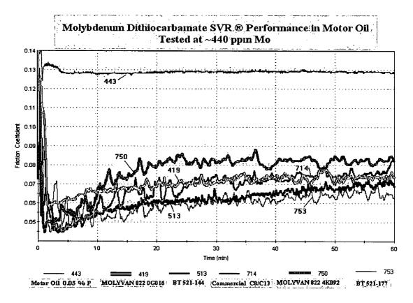
ASTM D5707: 200N; 50Hz; 80°C; 1H; 1mm Stroke; Ball on Disc
