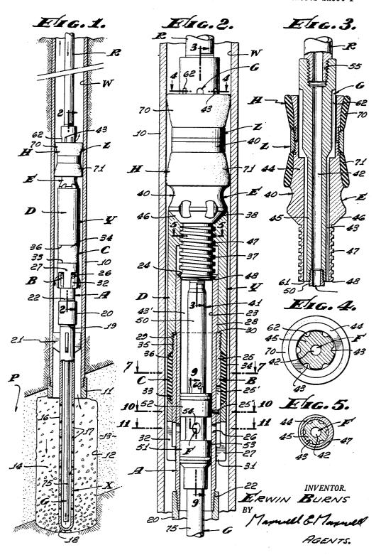
LINER AND GRAVEL PACKING APPARATUS FOR WELLS
