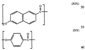
with said optional substitution if present being selected from the group consisting of an alkyl group of 1 to 4 carbon atoms, an akoxy group of 1 to 4 carbon atoms, halogen, and mixtures of the foregoing. The wholly 65 ety (XXIII), and approximately 5 to 45 mole percent of aromatic polyester there disclosed comprises approximately 10 to 90 mole percent of moiety (XIX) and approximately 90 to 10 mole percent of moiety (XX).
