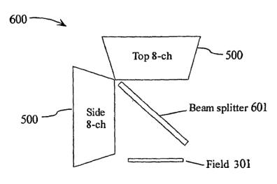
(57) Abstract: A imprint lithography system operable for imprinting a pattern into a material deposited between an imprint mold and a substrate, the system including, inter alia, a first set of imaging units positioned at a first angle relative to normal of the substrate; and a second set of imaging units positioned at a second angle relative to normal of the substrate, wherein the first and second angles are not equal to each other.
