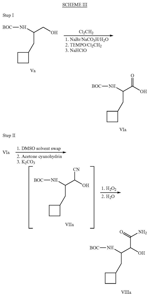
**[0037]** The process of the present invention utilizes a TEMPO mediated oxidation similar to that described in the '220 patent, however in the present invention process it is adapted to run in a dichloromethane reaction solvent instead of ethyl acetate. Although other solvents can be used, for example, ethyl acetate, it has been surprisingly found that dichloromethane is a suitable solvent for the TEMPO mediated oxidation which provides a clean reaction.
