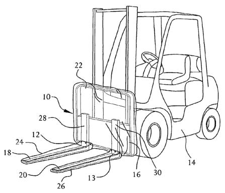
(57) Abstract: A protective covering to control the spread of contaminants associated with material handling equipment (14). The covering may comprise at least one sheet of a flexible substantially air tight material (22, 24, 26) adapted to enclose material handling equipment. The covering may also include collectors at specific locations to attract and collect contaminants raised by material handling equipment while running across a floor.
