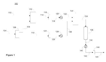
(57) Abstract: Provided is a process for the supercritical upgrading of petroleum feedstock, wherein the process includes the use of a start-up agent, wherein the use of the start-up agent facilitates mixing of the petroleum feedstock and water, thereby reducing or eliminating the production of coke, coke precursor, and sludge.
