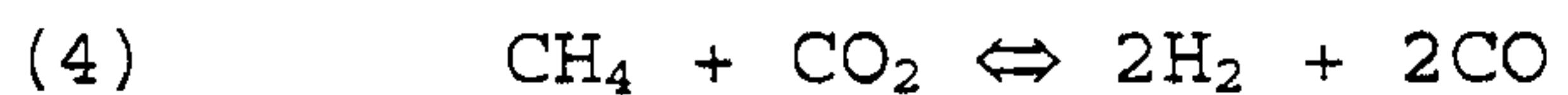
5 Combined steam and carbon dioxide reforming of hydrocarbons as illustrated below for methane:
