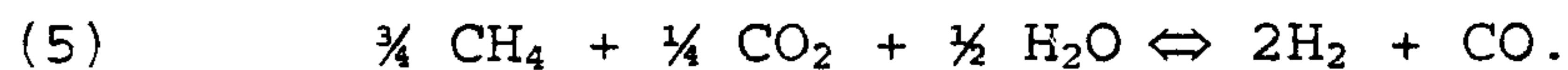
10 The ratio of steam to carbon dioxide can be varied to obtain the desired synthesis gas composition.
