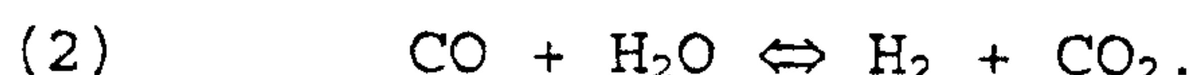
The above two reactions are in most cases close to equilibrium. If higher hydrocarbons (hydrocarbons with 2 or more hydrocarbon atoms) are present in the reformer unit feed stream, these are also steam reformed according to reactions similar to the above and as illustrated below:
