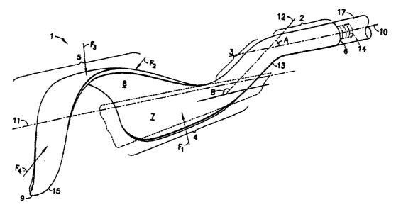
(57) Abstract: A handle support is constructed for removable attachment to, a tool, appliance or other implement for hand held use. The handle support includes a brace portion extending rearward in a helical form. The brace portion circumscribes an open space which is substantially conical in form.
