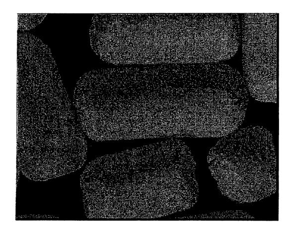
Lysine granule cores with starch
