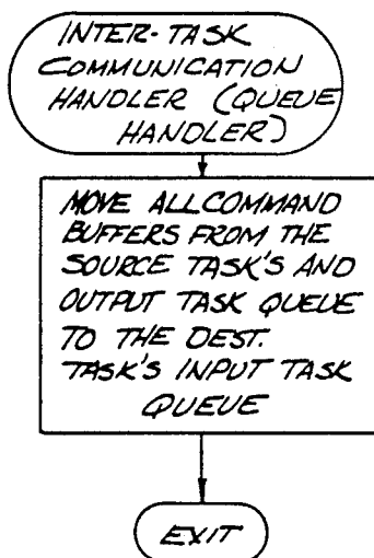
FIG. 9 INTER-TASK COMMUNICATION HANDLER
