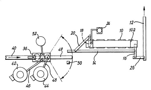
(57) Abstract: There is disclosed a process for treating sewage sludge or similar organic sludge in which dewatered sludge cake and an alkaline admixture are mixed and then dried under pasteurisation conditions utilising heat from the exothermic reaction with the alkali, in which drying is effected by extraction of moisture evaporated from the mixture by the exothermic heat.
