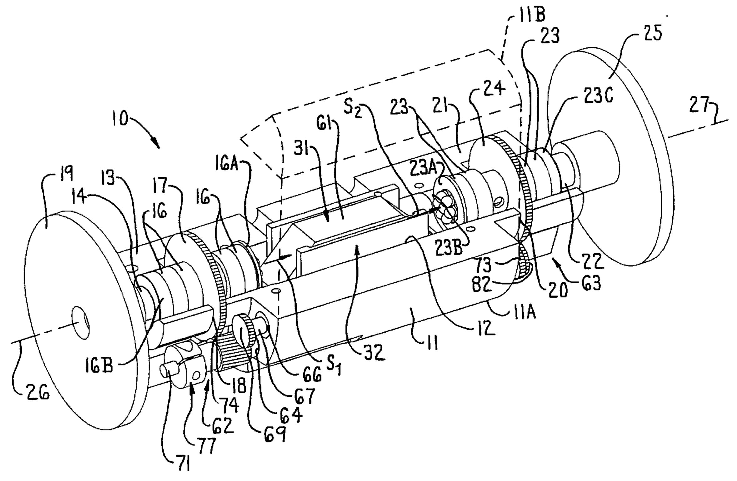
(57) Abstract: A multi-channel fiber-optic rotary joint having an elongate housing with a passageway extending therethrough. Fiber optic containing bundles are oriented in hollow shafts at the opposite ends of the passageway, which hollow shafts are rotatively supported in the housing. An alignment mechanism is provided inside the housing for effecting an optimizing of signal strength of signals transmitted between the respective fiber optic bundles.
