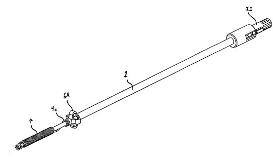
(57) Abstract: A device for inserting a stent in a body cavity, particularly useful for inserting a stent into a human male urethra to treat prostatic hyperplasia, whereby such device has an elongated member for removably receiving a stent and means capable of protruding from the member to either locate an obstruction, such as the sphincter muscle, in the body cavity or to prevent the stent from sliding off of the member, or both.
