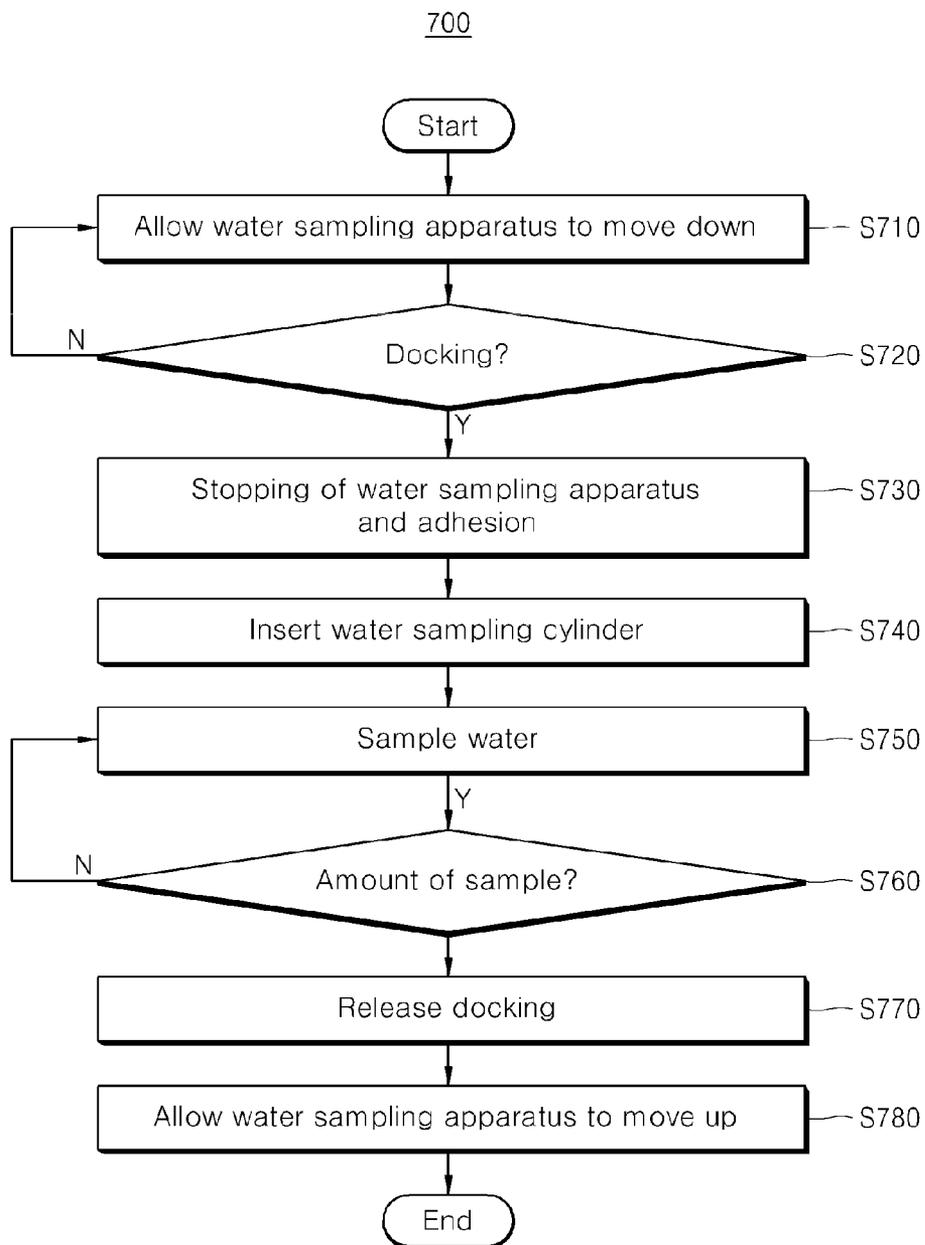
**APPARATUS FOR SAMPLING WATER IN BOREHOLE, AND METHOD THEREOF**
