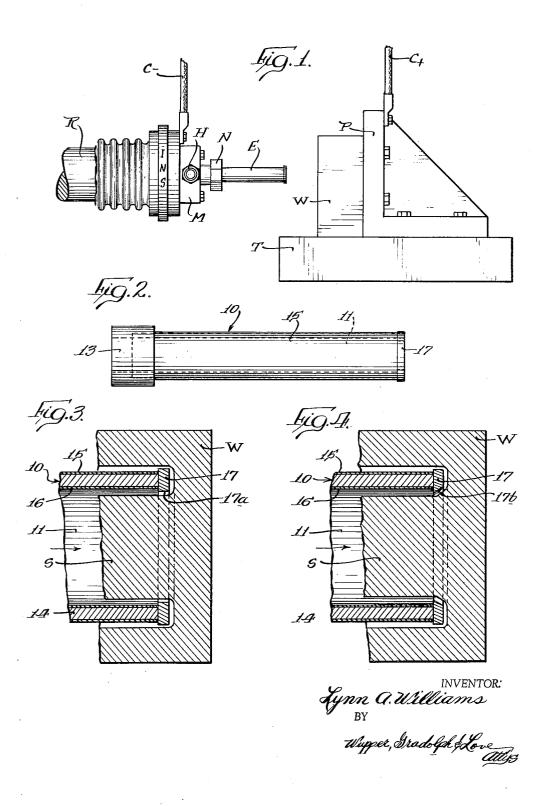
ELECTROLYTIC CAVITY SINKING APPARATUS AND METHOD
