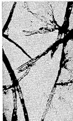
Prehydrolysis sulfate softwood pulp with 7% NaOH solution extraction
