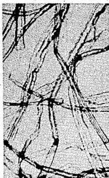
Prehydrolysis sulfate softwood pulp, with no concentrated caustic extraction
